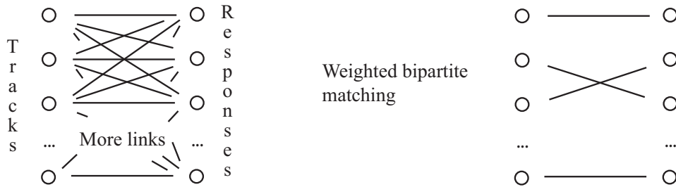
FIGURE 1.1: In tracking by detection, we must associate detector responses in the current frame with tracks carried over from the previous frame. We compute a weight for associating a particular track with a particular detector response; this weight could involve information about how fast objects are expected to move, and about the appearance of the response. Large weights are good and small weights are bad. We must choose the matching that has the largest sum of weights. This is a maximum weighted bipartite matching problem, where the one side of the bipartite graph is the tracks and the other is the responses. A new track is created for any response not matched to a track. Tracks that are not matched to responses for several frames are dropped. In some cases, it is useful to attach null tracks and null responses with a fixed association weight, to encourage tracks to be unmatched.
